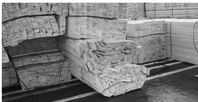
Figure 6.2. Example of poor rigidity
