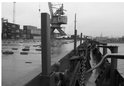
Figure 6.7. Example of uprights for bottom blocking
